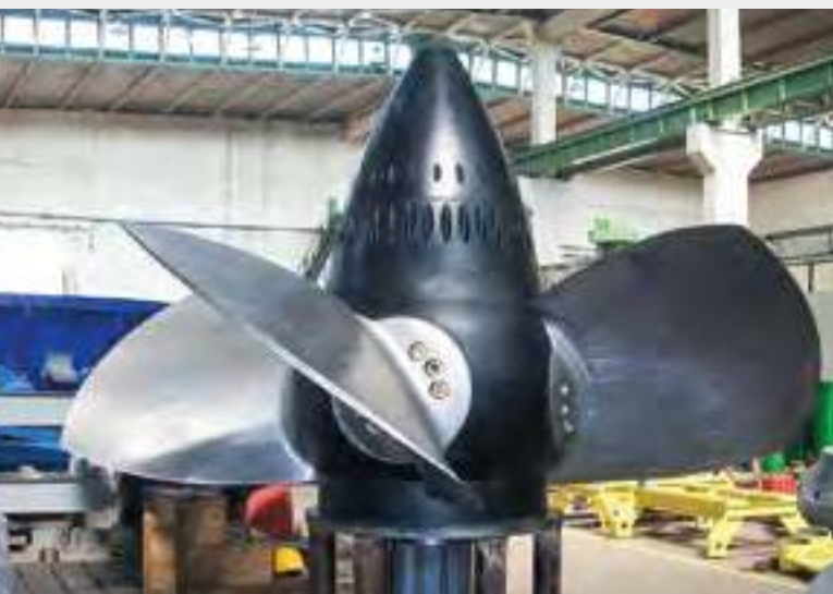
Akinci - I/II, Turkey Type of Turbines: 'PIT' Type – Axial Flow Rated Head: 6.40 m Installed Capacity: 4 x 3,600 kW
