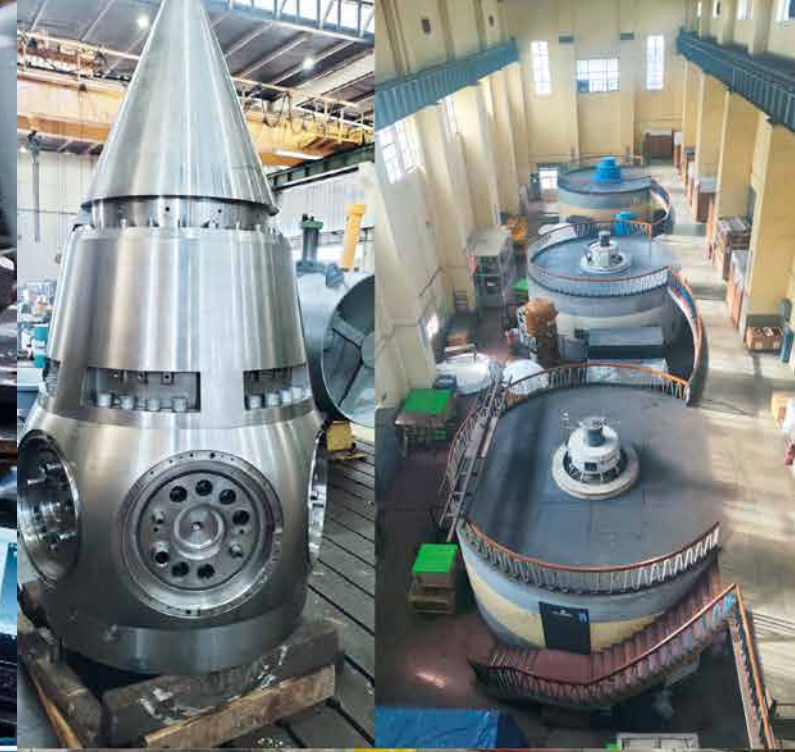
Koyna, Stage II, HEP, India Type of Turbines: Vertical Pelton Rated Head: 490.00 m Installed Capacity: 2 x 80,000 MW
