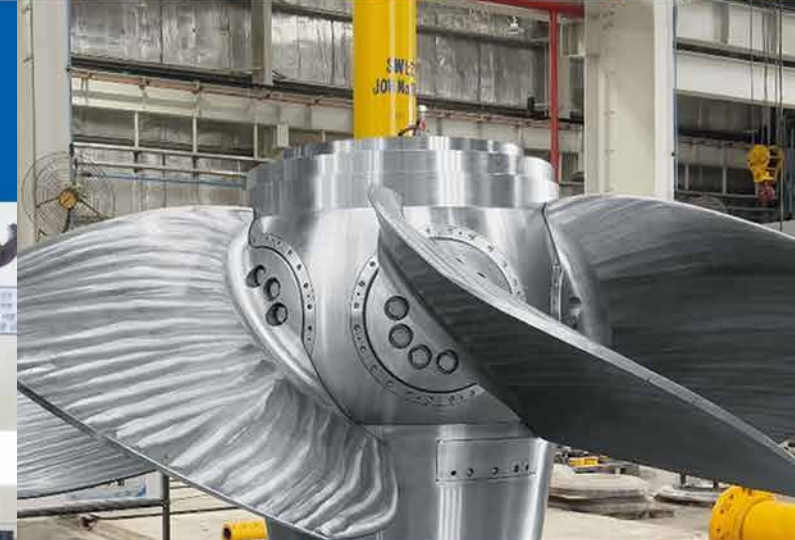
Dhokrani HEP, India Type of Turbines: Vertical Full Kaplan Rated Head: 19.60 m Installed Capacity: 3 x 11,250 kW
