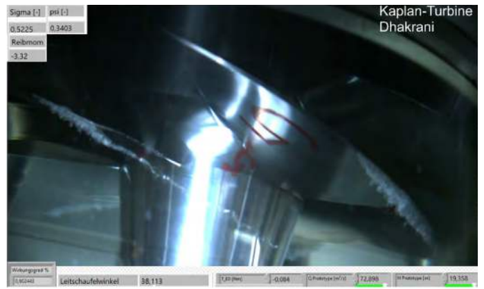
Figure 111: Cavitation behaviour for \sigma_{PLANT} = \sigma_0 , H_p = 19.6 m, Q_p = 73.0 m³/s, \beta = 10.0^\circ
